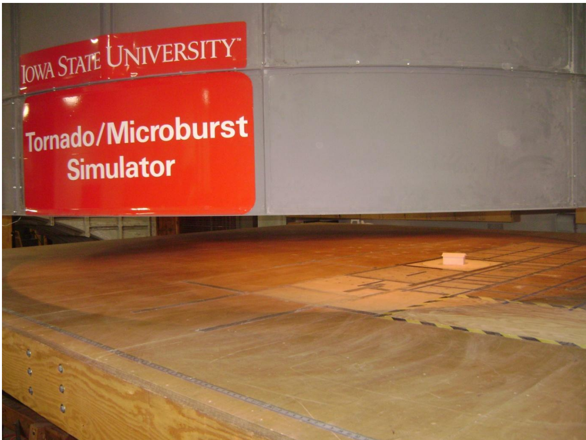
FIGURE 2-1 ISU TORNADO SIMULATOR WITH LOW-RISE BUILDING MODEL
